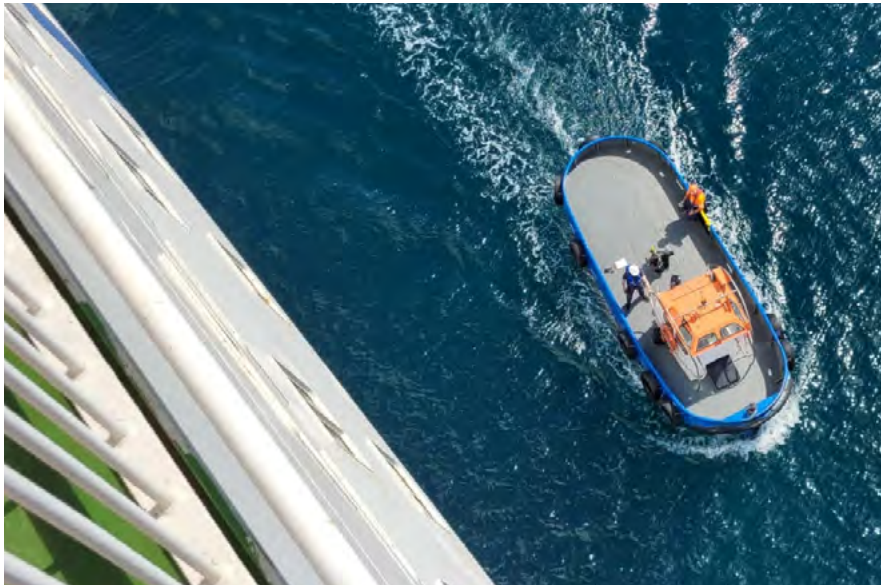
Onboard launch to read draft marks: Tymor Marine MD Kevin Moran and Principal Naval Architect Niall MacLennan travel by launch to capture draft readings as part of the lightweight survey aboard Global Mercy.
