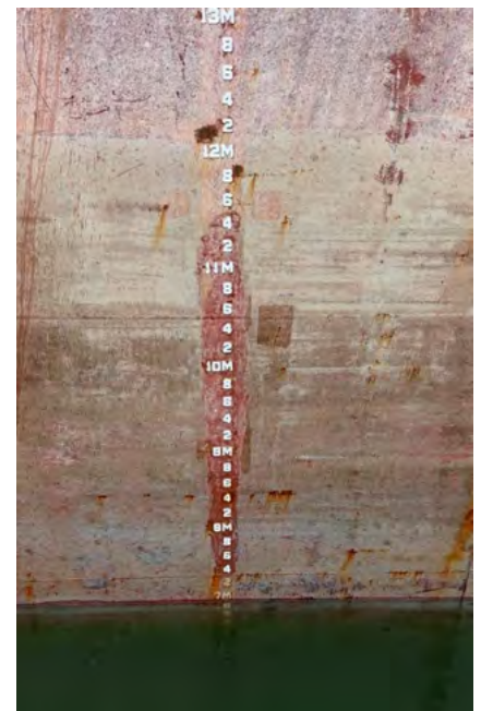
One of the draught measures on the side of the coal ship.
