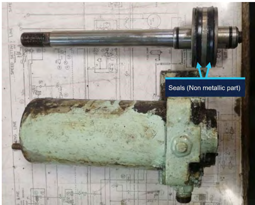
Figure 5: Main air distributor reversing cylinder/servo piston with new seals. Note: The image shows the piston after the seals had been replaced. (Source: Ship's manager, annotated by the ATSB)
